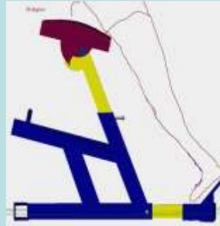
↑ 30 degree pad angle placement as shown above.
